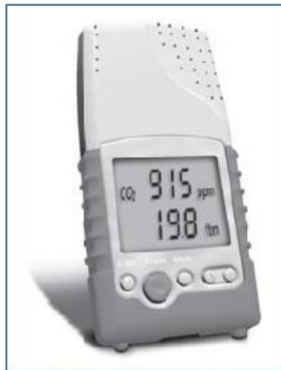
Figure 2. Typical non-dispersive infrared spectroscopic CO 2 sensor.
